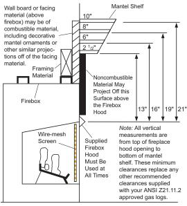
Figure 18 - Minimum Mantel Clearances for Built-In Installation
